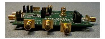
Objective: To band-shift the RF matching from the U.S. to the Japanese cellular band, and to measure the performance of this CDMA dual-mode front-end IC.
